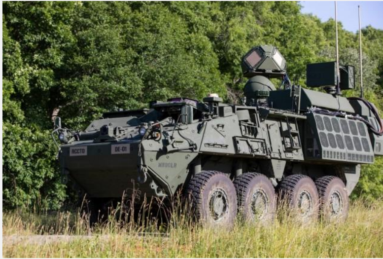
Figure 1: Directed Energy Maneuver Short-Range Air Defense (DE M-SHORAD) 50 kW-class laser weapon system mounted on a Stryker A1 8×8 armored vehicle. The roof-mounted beam director turret, internal laser and power-thermal management system (PTMS), and Ku-band AESA (Active Electronically Scanned Array) radar are visible. Source: U.S. Army Rapid Capabilities and Critical Technologies Office (RCCTO), image via Defense Visual Information Distribution Service (DVIDS). Public domain.
