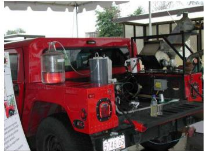
Water recovery from engine exhaust by Lexcarb LLC and U.S. Army TARDEC
